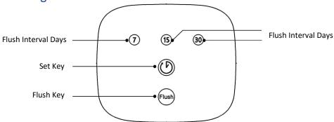
**Power first supplied:** system beeping meanwhile lights are flashing, with the five lights flashing simultaneously for one time, system enter the factory default setting(15 days), if there is no other operation, system enters sleep mode in 8 seconds.
